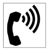
Figure 703.7.2.3 Volume Control Telephone
