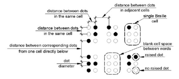
Figure 703.3.1 Braille Measurement
